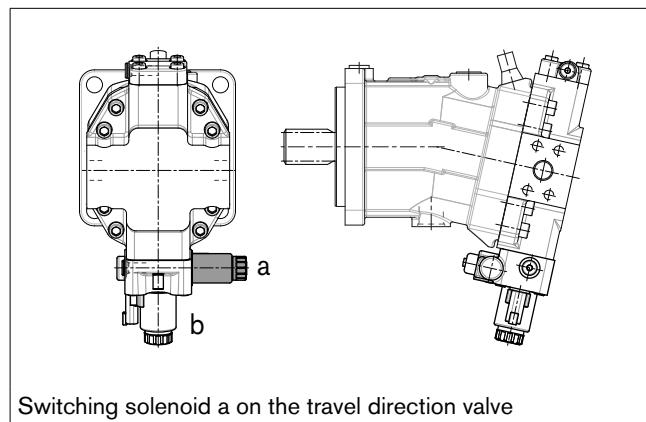
Switching solenoid a on the travel direction valve
