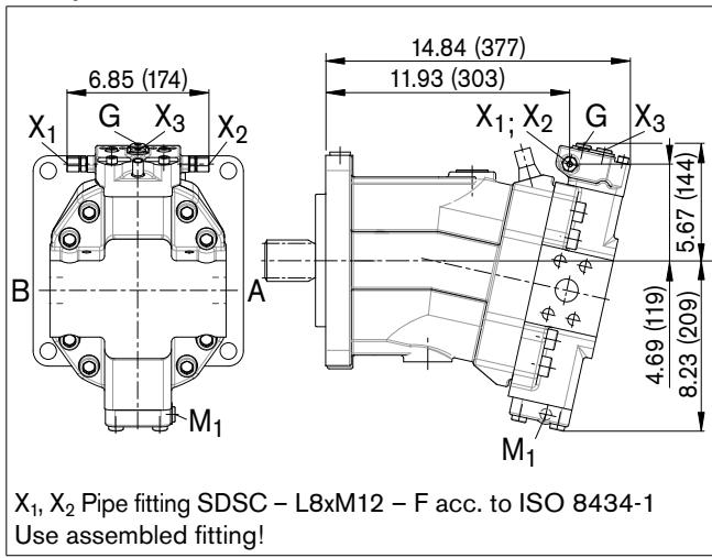
X<sub>1</sub>, X<sub>2</sub> Pipe fitting SDSC – L8xM12 – F acc. to ISO 8434-1
