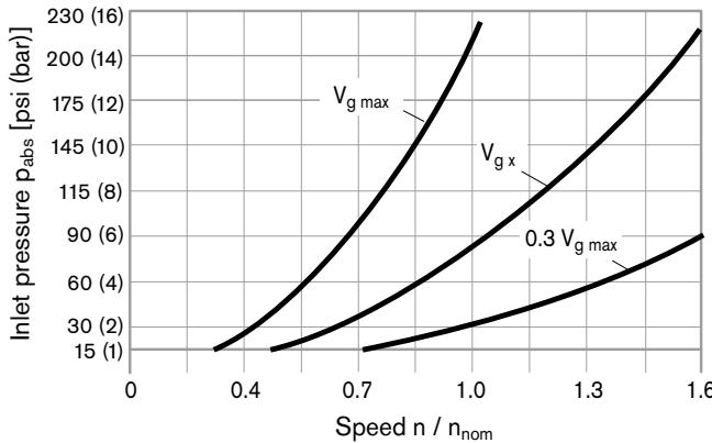
This diagram is valid only for the optimum viscosity range from  $\nu_{\text{opt}} = 170$  to 74 SUS (36 to 16 mm<sup>2</sup>/s).
