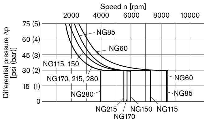
The values are valid for an ambient pressure  $p_{abs} = 15$  psi (1 bar).
