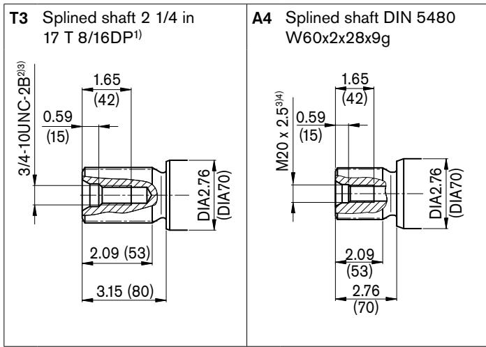
1) ANSI B92.1a, 30° pressure angle, flat root, side fit, tolerance class 5
