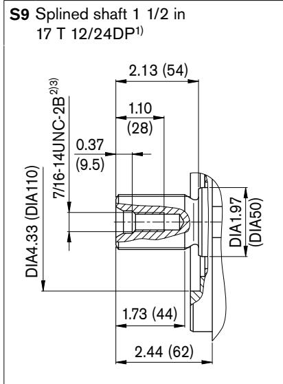
1) ANSI B92.1a, 30° pressure angle, flat root, side fit, tolerance class 5
