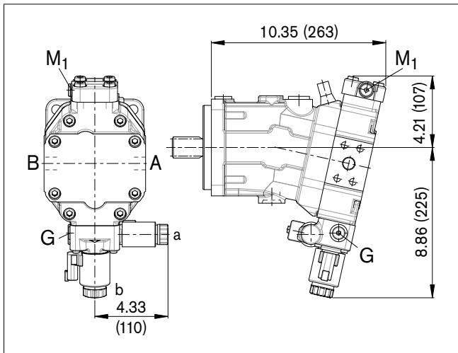
Before finalizing your design, request a binding installation drawing. Dimensions in inch (mm).
