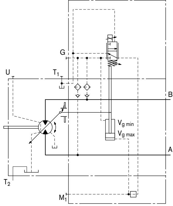
Schematic EP1, EP2: positive control
