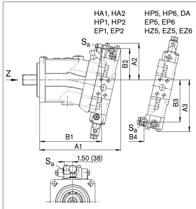
Dimensions of size 115 (medium flushing valve)
