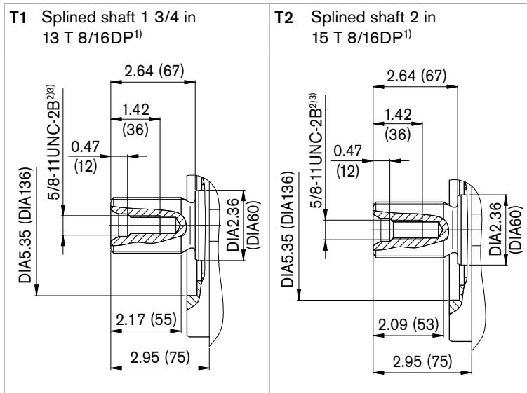
1) ANSI B92.1a, 30° pressure angle, flat root, side fit, tolerance class 5
